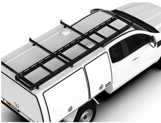
PIPE RACK W450 x L3200mm
