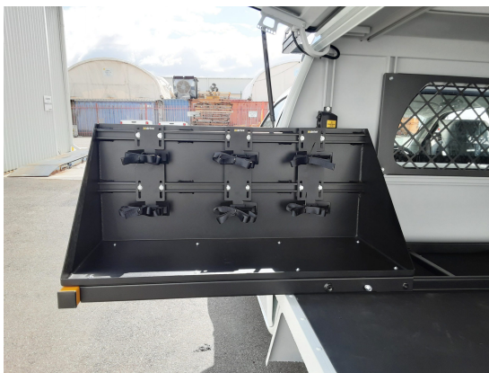
SIDEWAYS GAS BOTTLE SLIDE W460 x L640mm
