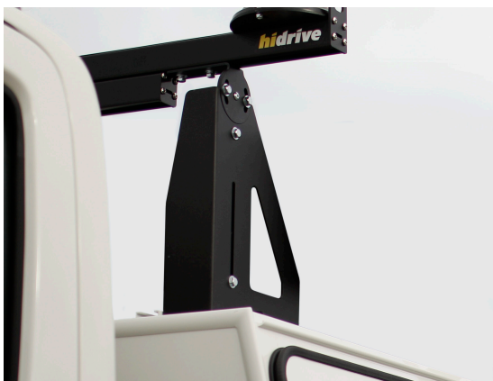
ROOF BAR RISER Rear
