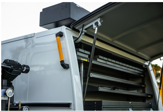
GRAB HANDLE, FITTED TO BODY (TRUCK) 300mm, safety yellow
