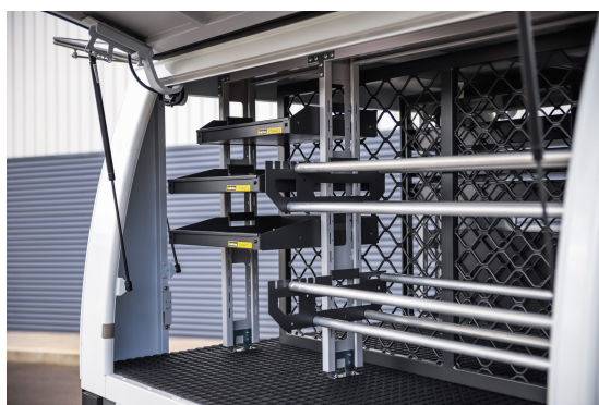
ONE-CLICK ADJUSTABLE CABLE REEL HOLDER (TRUCK) L920mm
