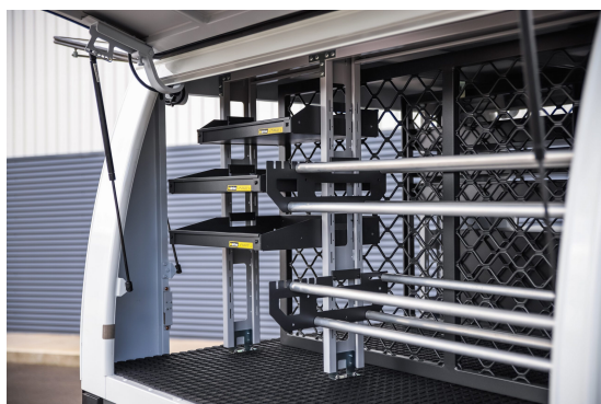
ONE-CLICK ADJUSTABLE CABLE REEL HOLDER (TRUCK) L690mm
