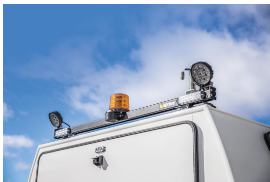
MINE BAR WITH LED BEACON L1375mm bar
